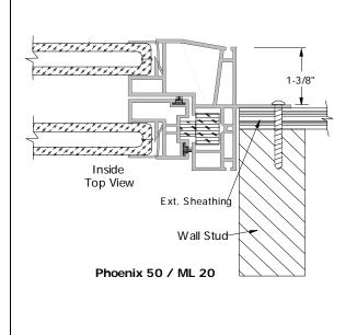
Note: We strongly recommend the use of flashing and/or flashing tapes and sill pans as stated in ASTM E 2112-01. However, due to variation in codes and building types, it is left up to the end user to determine the proper installation of these items.
